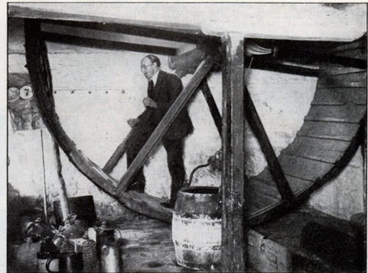
Fred Hoare, of Beauworth, England, is drawing his daily supply of drinking water. He does this by taking his exercise inside the twelve-foot treadmill which winds up a cable from the well
